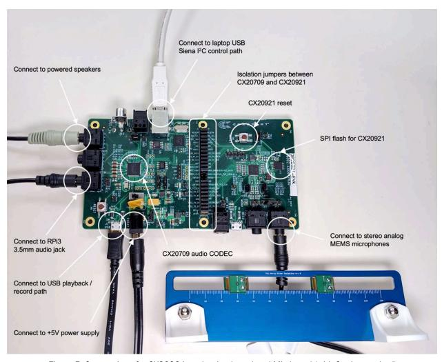
Figure 5. Connections for CX20921 evaluation board and Mic board (with 2-mic attached)
