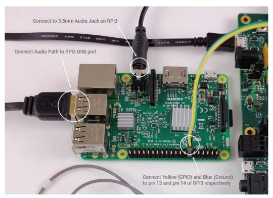
Figure 6. Connections for RPi3
