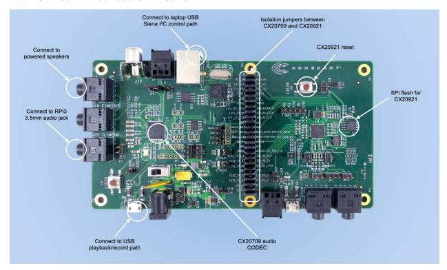
Figure 2. CX20921 Evaluation Board: Connections, Interfaces and Devices
