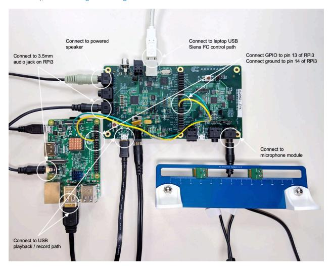
Figure 4. CX20921 evaluation board setup with RPi3 board and Mic board (with 2-mic attached)
