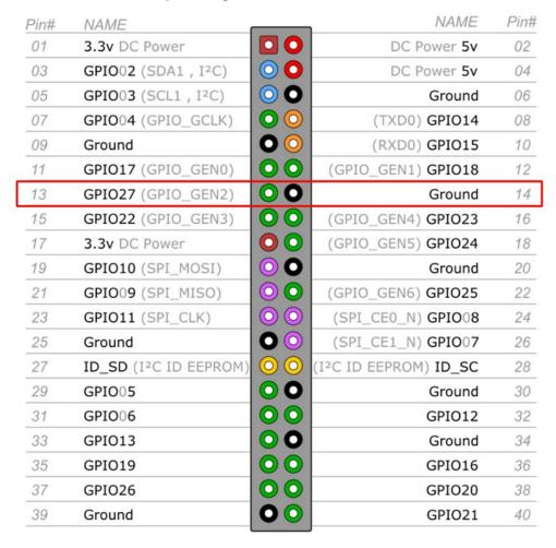
Figure 3. RPi3 pinout
