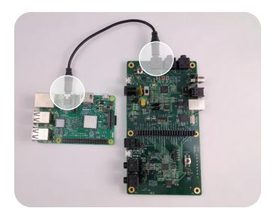
Connect the 3.5 mm audio jack on the RPi3 (J7) to LINE IN on the CX20921 evaluation board (J25).
