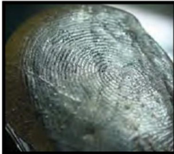
Figure 1: Fake finger cast with ordinary wood glue and coated with graphite powder
